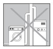
Note that to avoid condensation problems, it is essential that the dryer be fitted with the flexible hose to carry its "exhaust" at least beyond the kitchen units; preferable outside the kitchen.
